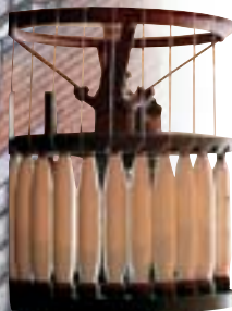
▲ Bobbins with machine-spun thread
